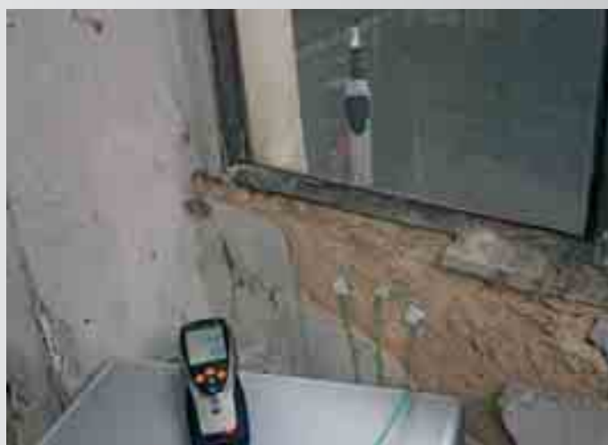
Measuring the U-value at a wall in need of repair with a U-value and wireless temperature/humidity probe (also possible with a temperature probe)
