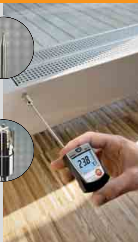
Checking temperature on a radiator
