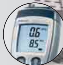
Simultaneous display of flow and pressure value
