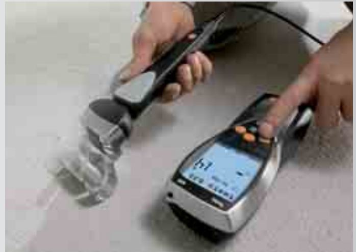
Determining screed moisture quickly and easily. Measuring several points over a surface with the scatter field probe ensures better security of measurement.
