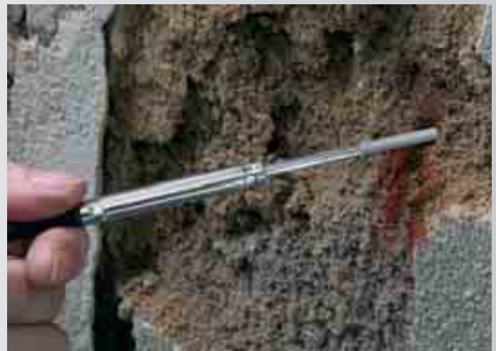
Inserting the humidity probe in a bore hole with PTFE protective cap
