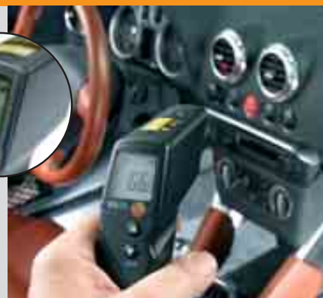
Checking temperature at a ventilator
