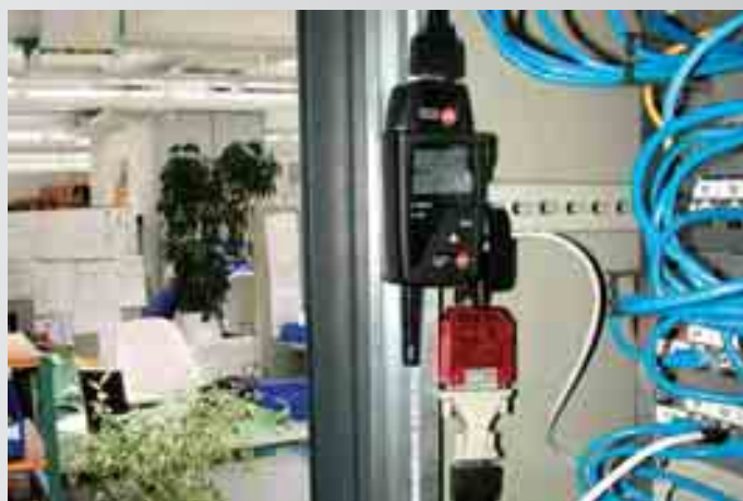
Read out the data stored in the logger via the PC network using the Ethernet adapter
