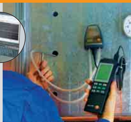
Pitot tube measurement with external 100 Pa probe
