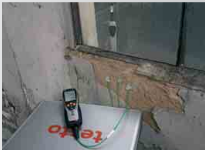
Measures the U-value in a wall in need of renovation using U-value and wireless temperature/humidity probe (alternatively conventional temperature probe also)
