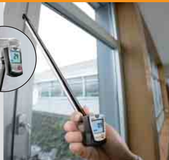
Flow velocity measurement at nontight windows
