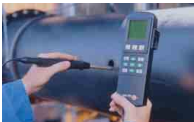
Humidity measurement in a bio-filter. Advantage: Accurate measurements in the high humidity range or in temperature fluctuations, without condensation on the probe which cause incorrect measurements.
