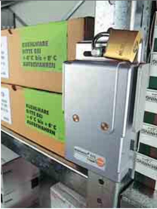
testostor 171-0 monitors fluctuations in temperature constantly
