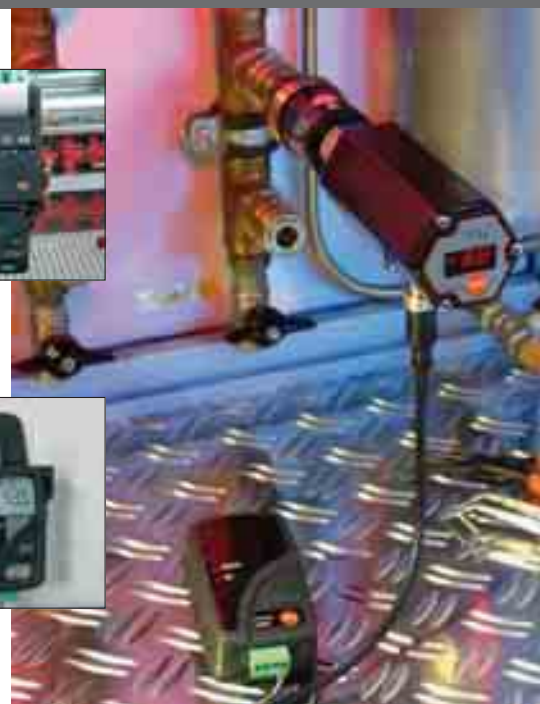
Recording the current of a measurement transmitter with testo 175-S1 (without display)
