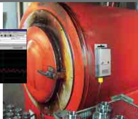
Monitors temperatures in a hardening furnace
