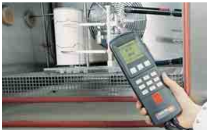
Measurements in climatic cabinets with the highly accurate reference humidity/temperature probe. Advantage: accurate monitoring of fluctuations in air humidity with an accuracy of \pm 1\%RH
