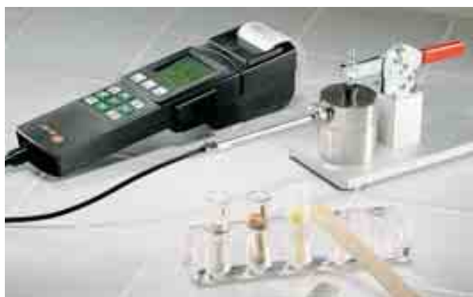
Quality control monitoring of pharmaceuticals. Advantage: Results are traceable to national standards. testo 650 automatically indicates when a sample reaches equilibrium, signalling the end of the test. Constant monitoring is therefore not required. Calibration on location with control and adjustment set, with DKD calibration certificate if required. Advantage: This provides additional quality assurance.
