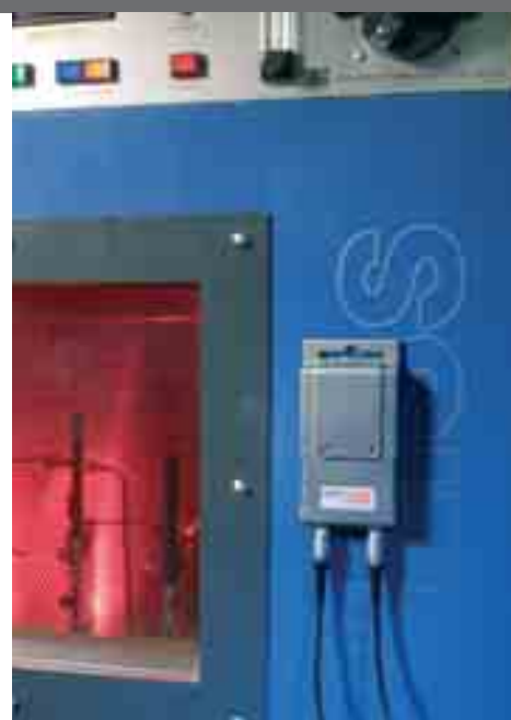
Monitoring air humidity/temperature fluctuations in climatic cabinet
