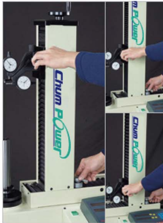
X and Z axes are equipped with precision linear guideways, allowing for rapid traverse and micrometric transmission. X、Z軸附精密線性滑軌，可做快速移位及微調傳動。
