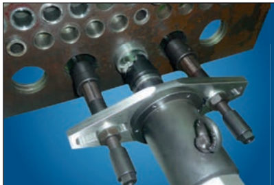
⚙ Reducing tube wall on a 6" thick tube sheet prior to punching.
