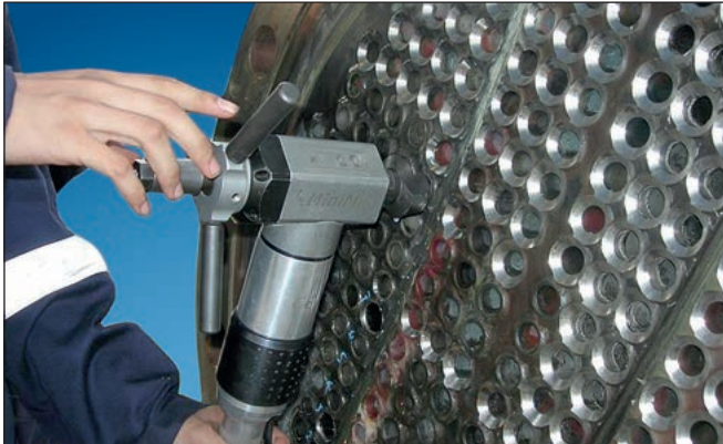
☞ Strength weld removal on 1" x 12 MW tubes, leaving a perfect weld prep for re-welding once tubes have been removed. Speed reducer recommended.
