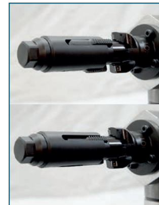
Custom machined jaws. Showing locked and up-locked position.
