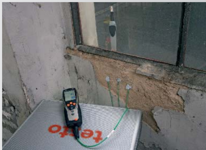
Measures the U-value in a wall in need of renovation using U-value and wireless temperature/humidity probe (alternatively conventional temperature probe also possible)
