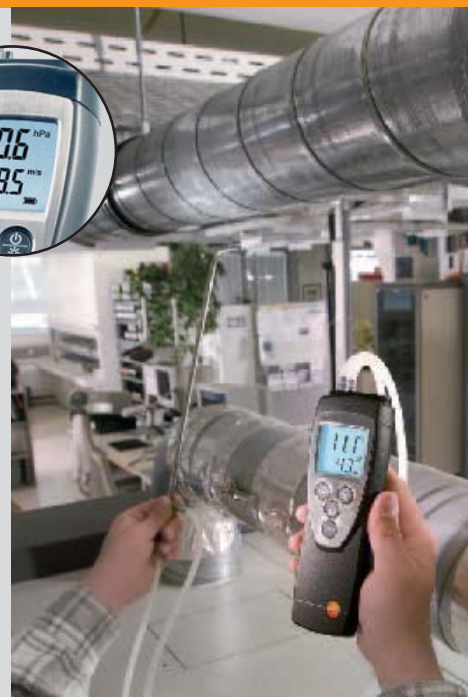
Measuring process air
