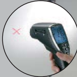
Switchable optics 1: far field 75:1 (16 mm, 1200 mm distance) with cross-laser sighting
