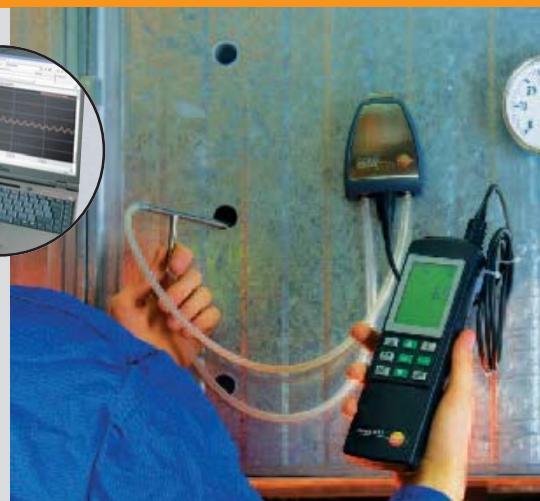
Pitot tube measurement with external 100 Pa probe
