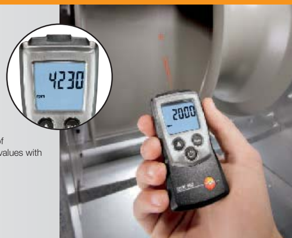
Non-contact rpm measurement on a ventilator
