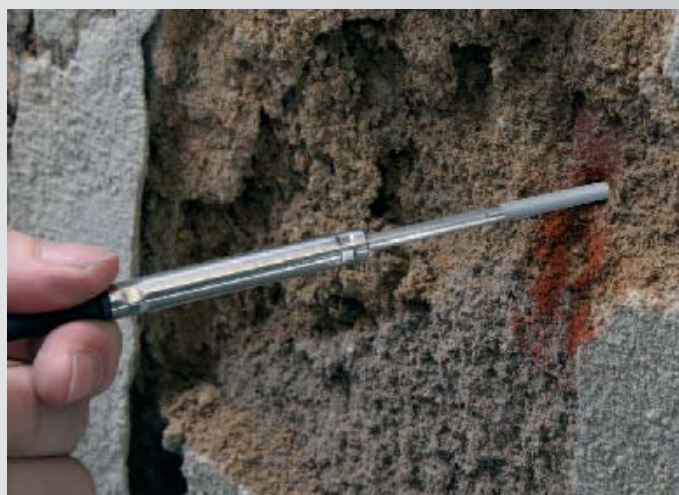
Inserting the humidity probe in a bore hole with PTFE protective cap
