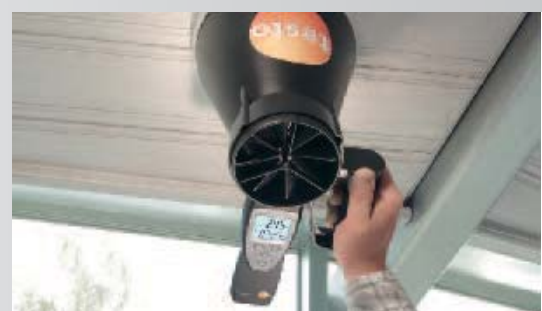
Monitoring ingoing air in a disc outlet
