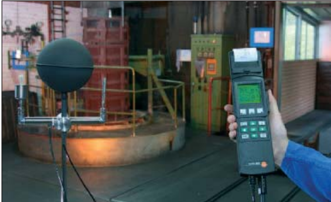
Measure with testo 400 and WBGT probe
