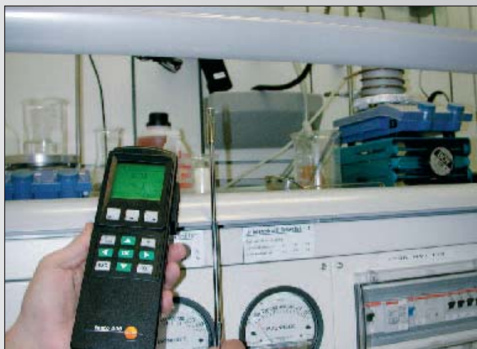
On-site testing of a laboratory fume cupboard with testo 400
