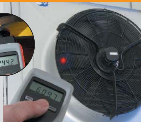
testo 465 and testo 470, non-contact (optical) rpm measurement on rotating parts
