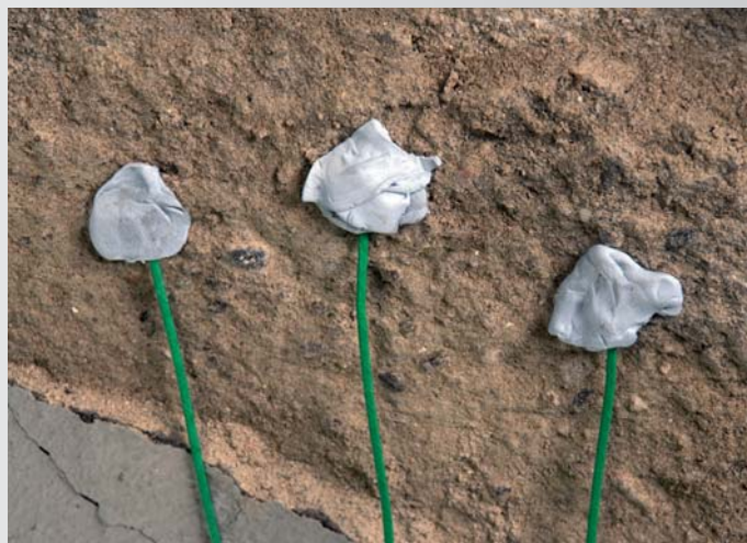
Measures wall surface temperature using three fast-action thermocouple sensors
