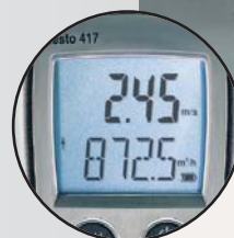
Volume flow is shown directly in the large display
