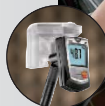
Monitoring air humidity, e.g. in an air conditioning duct
