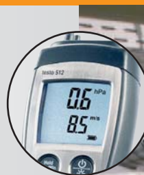
Simultaneous display of flow and pressure value
