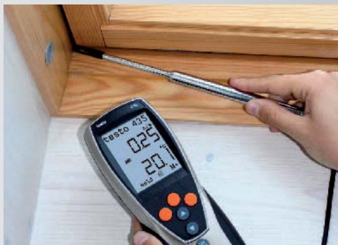
Measuring flow at a leaking window
