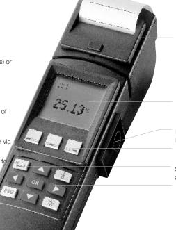
Attachable printer Prints readings on site in the matter of seconds
