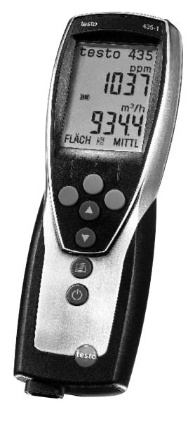
testo 435-1, multi-functional meas. instr., for A/C, ventilation and Indoor Air Quality, with battery and calibration protocol
