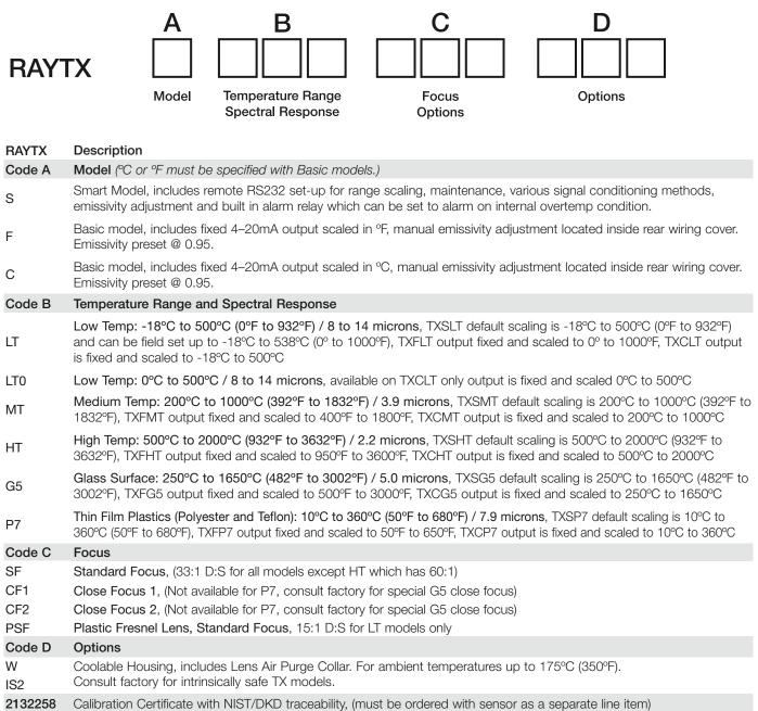
Included with each sensor is a mounting nut, a fixed mounting bracket and an operator's manual. Typical Model Number: RAYTXSLTSF Specifies a Smart, Low Temperature, Standard Focus, TX sensor
