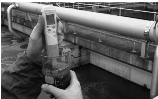
Figure 23: pH range in the biological stage of waste water treatment
