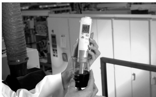
Figure 24: pH value of developer in a large photo laboratory
