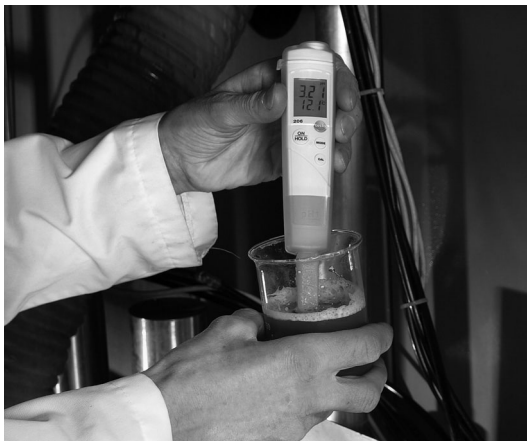
Figure 27: pH value during the manufacture of fruit juice
