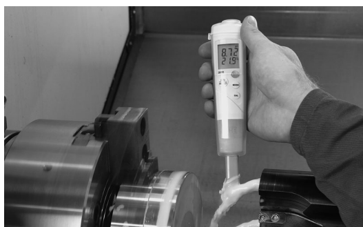
Figure 25: Determining the pH value of the lubricating and cooling membrane in a turnery
