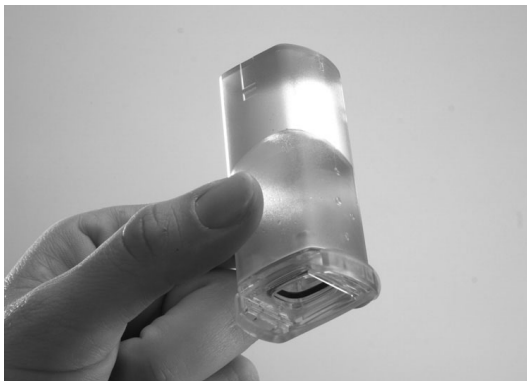
Figure 32: Storage cap for pH probes with spill-proof KCL gel
