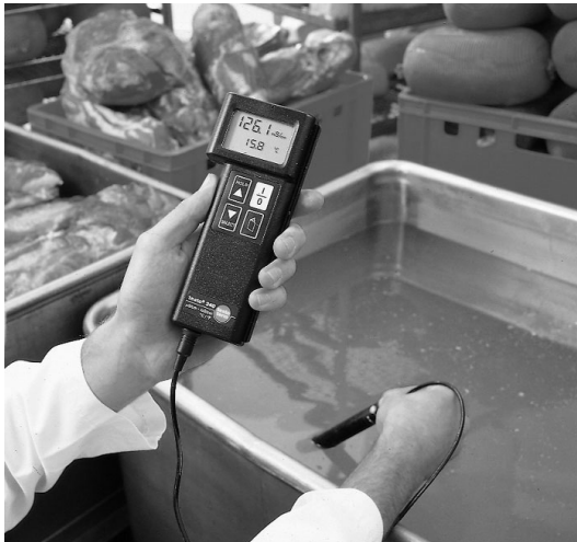
Figure 31: Measuring conductivity in the brine during the processing of ham
