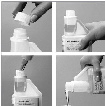
Figure 16: Easy and fast calibration using a calibration reservoir
