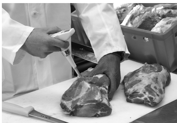
Figure 20: pH measurement in the meat producing industry
