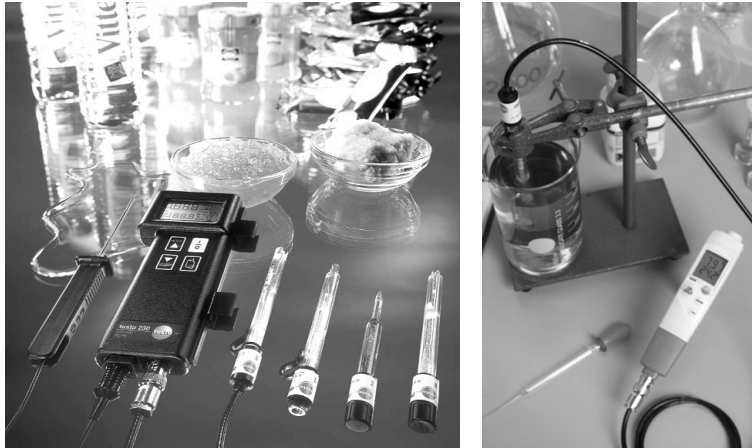
Figure 3: Example of a pH measurement system with separate measurement probes (testo 230 with pH probe and stainless steel temperature probe and testo 206-pH3).
