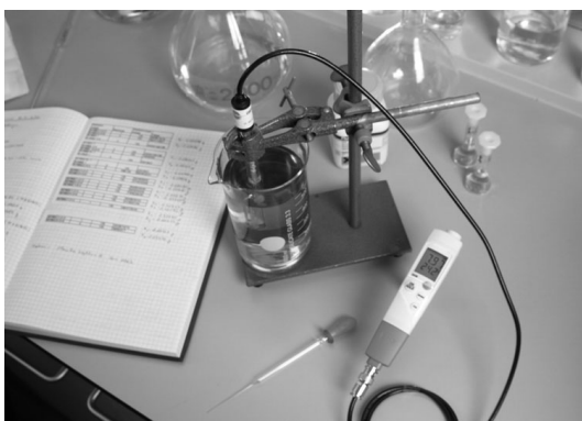
Figure 29: pH value check in laboratories
