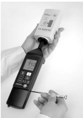
Figure 17: Calibrating testo 815/816 with a calibrator
