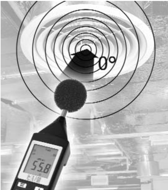
Figure 15: Positioning of the microphone according to DIN/IEC
