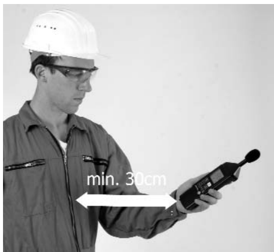
Figure 16: Handling the microphone
