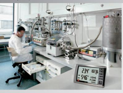
A glance at the testo 622 is enough: up-to-date temperature and humidity values as well as date and time can be read out immediately. In addition to this, the measuring instrument can be calibrated and adjusted with the help of the calibration and adjustment software – that saves time and costs.
