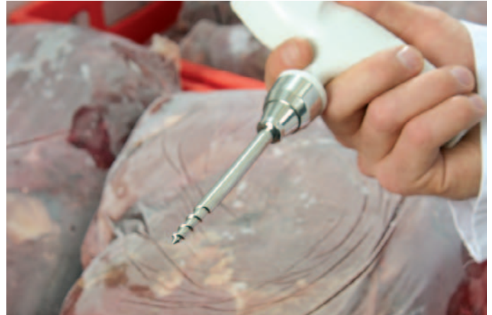
testo 105 with frozen food probe, core temperature measurement without pre-drilling
