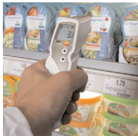
2-point laser shows the exact measurement spot.
