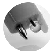
pH1 probe head for liquids
