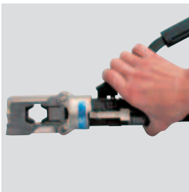
EP-50 (One hand operation to hold connector)
